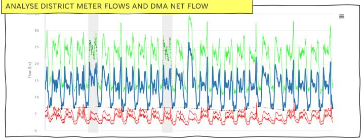
Let me check the flows for each alarmed DMA: every **district meter flow** is shown, inflows are green, outflows are red and the **calculated net balance** is blue. Missing data are interpolated from the past and the minimum night flow is identified.
